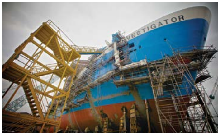
The 93.9 metre Investigator when it was under construction. Image courtesy of CSIRO (CC BY 3.0)
