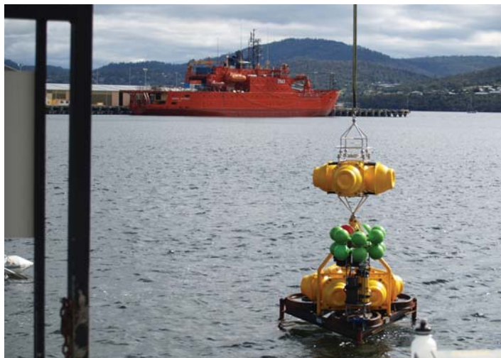
Testing components of a mooring at CSIRO, Hobart. The mooring will be one of three deployed from the Aurora Australis (behind) this month in the Southern Ocean near the Mertz Glacier. The data will be retrieved in two years. Photo courtesy of CSIRO
